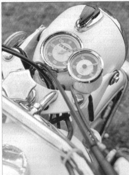
Control layout, with speedometer mounted in headlight and rev-counter on separate bracket.
